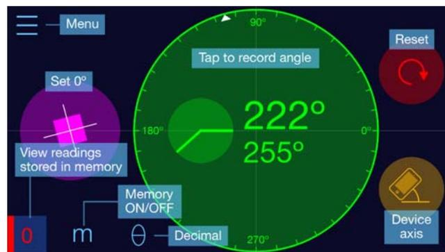
Figure 10: Application “G pro” for the iPhone 5 to measure range of motion in the SLR test
